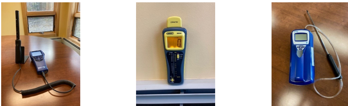
Figure 5: TSI Q-Track IAQ Monitor, General Moisture Meter, TSI P-Trak Ultrafine Particulate Counter
