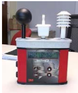
Figure 2: Quest Wet Bulb Globe Thermometer used by OEHS to monitor weather for health advisories
